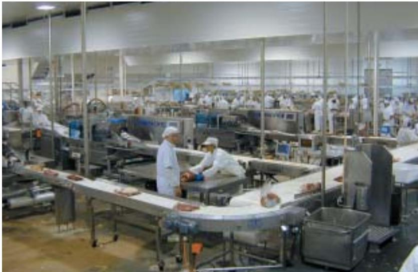
■ ULMA Packaging recently installed three fully automated vacuum packaging lines at Richmond ND's packaging plant in Whakatu (New Zealand), all of which have been integrated into the facility's production system. The first fully automated line in the world it will be used to process cuts of beef and has a processing capacity of 650 cows per shift. Each line can package 50 packs per minute. New innovations mean considerable savings in packaging material, a sizeable increase
