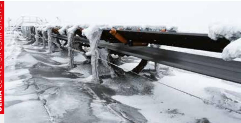
stopped. This avoids frozen liquid blocking the rotation of the roller and ensures that start-ups of conveyors in sub-zero conditions are not problematic.
