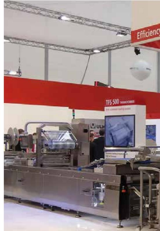
sanitizable design and an Elcat autoloader for sliced products. A thermoformer with side extraction of the moulds which allows the format changes to convert into a quick and easy operation.
