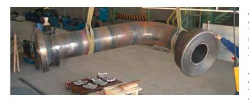
ULMA Piping has obtained its first large order of alloy-coated, corrosion resistant Spools.
