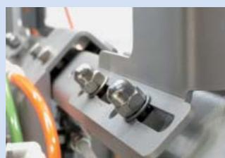
Separated surfaces to avoid the accumulation of residues.
