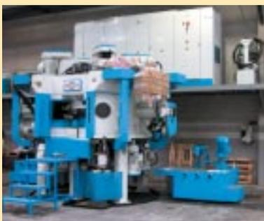
The first week of October, a new Transfer machine for the Mechanization of Forged Fitting arrived at ULMA Forging from Gnutti, in the north of Italy. This machine will specialize in the complete mechanization of elbow and " T " couplings from 1 up to 2 NPT and
