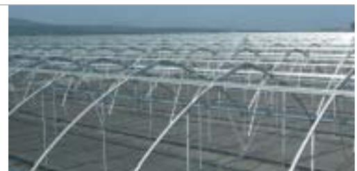
ULMA Agrícola is executing various large-scale projects in Mexico. It is currently finalizing one of the most complete facilities made since its presence in Mexico. The greenhouses are a G8 model Gothic Multispan type, 4.5 m below the channel, equipped with a butterfly model top ventilation while the sides and fronts roll up and down. All ventilation is motorised and have the openings protected with a 10x16 and 16x20 anti-aphid mesh. These facilities have various
